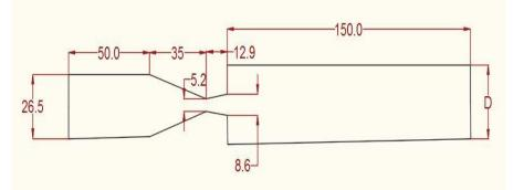
Fig.1: Dimensions of nozzle and enlarged duct
