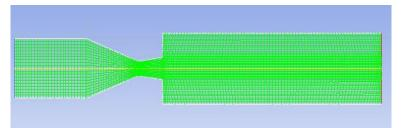
Fig.2: Meshed model of nozzle and enlarged duct
